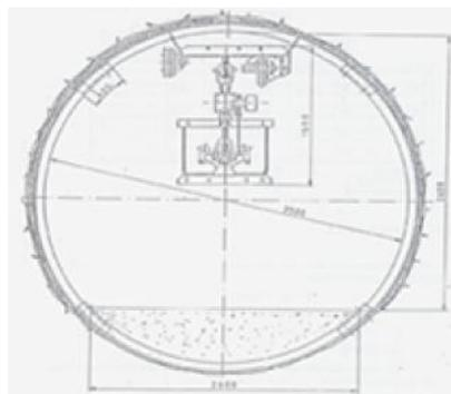
**Figure 1. Cross section of room with ropeway elements**
