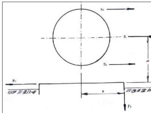
**Figure 3. Action of force on foundation of the driving machine**
