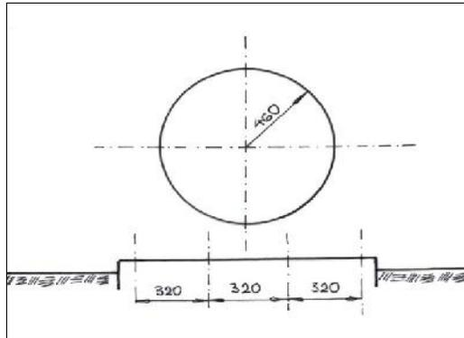
**Figure 2. The foundation of the driving machine**
